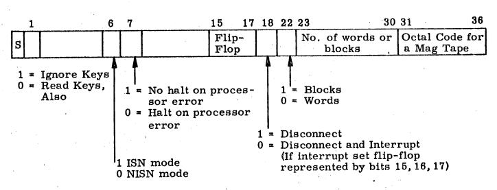
Read data from a magnetic tape according to the code word into location DATA and following.
