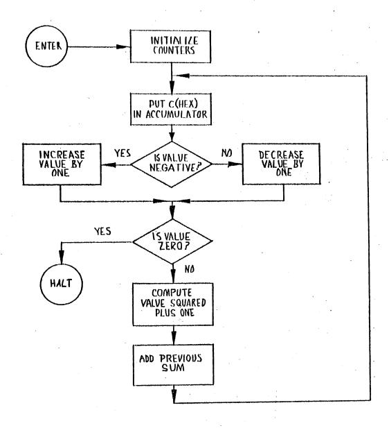
4.2.2 x is a non-zero integer stored in location HEX. Test to see if x is positive or negative. If positive, decrease it by 1; if negative, increase it by 1. Now compute x<sup>2</sup> + 1 for every integral value of x from the present value of x to, but not including, zero at which time halt the machine. Keep track of the number of times x is computed in location SUMA. Store the total sum in location SUMB
