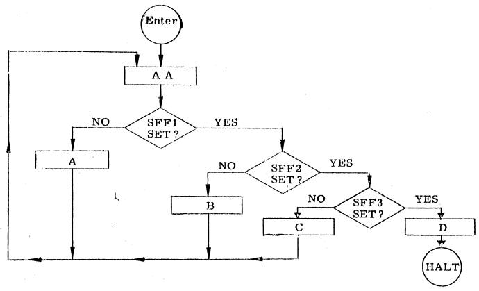
Alternate the program so that the first loop goes through A, the second through B, the third through A, the fourth through C, the fifth through A, the sixth through B, the seventh through A and the eighth through D. Assume no flip-flops are set initially. Be concerned with the sense instructions only.
